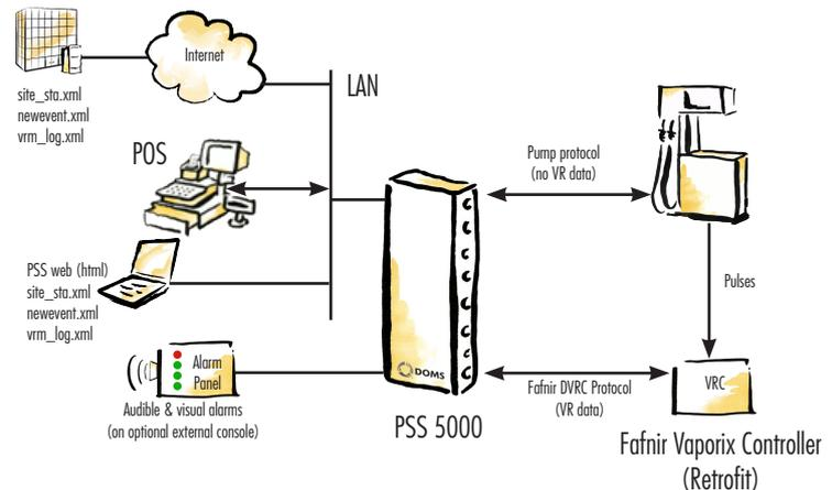
In this scenario, the communication protocol between the PSS 5000 and the dispenser does not support vapour recovery error data. However, the VRC is connected directly to the PSS 5000 and communicates with a protocol that supports vapour recovery data.
