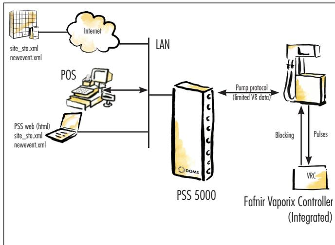
It is the integrated VRC that hosts the VRM<sup>1</sup> rules and controls all this functionality. The VRC registers any malfunctions in the vapour recovery system, triggers and elicits the necessary alarms and is responsible for blocking the fuel being dispensed so long as the VRM rule violations are not rectified.
