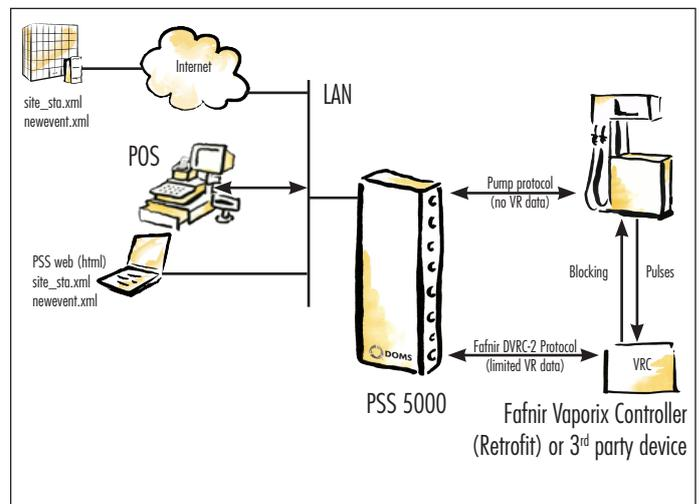
The VRC is configured using the Doms POS installation parameters. These are used to assign the VRC to the fuelling point(s), and it is the VRC that blocks the dispenser when the VRM<sup>1</sup> rules are violated.
