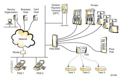
In this scenario, the PSS 5000 controls the operations of the forecourt pumps, price poles and payment terminals, and provides a generic interface to the Tank Gauge System for a readout of inventory data and deliveries. The PSS 5000 also ensures that any price changes are shown correctly on both the pumps and price poles.
