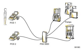
In this scenario, the PSS 5000 is used to control the fuel pumps and connect to the Point-Of-Sale (POS) terminals. Payments for the transactions take place via the POS terminals.
