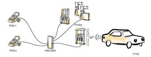
In this scenario, the vehicle is identified using a vehicle inlet tag, which is read by the nozzle reader. When a valid tag is presented, the PSS 5000 is able to authorize the dispenser to start. If the connection between the vehicle tag and nozzle reader is broken, then the dispenser stops the fuelling until the two are reconnected. Payments for the transactions take place via the POS terminals.
