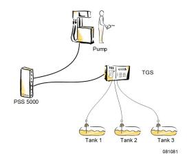
In this scenario, the PSS 5000 is used to provide transaction data to the Tank Gauge System (TGS) so it can verify that all the wet stock movements are legitimate.
