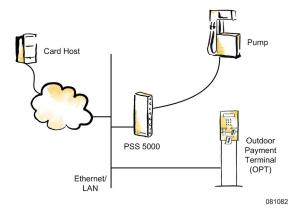
In this scenario, the PSS 5000 is used to control the fuel pump and authorization is controlled via a 3rd party payment solution for cards and/or bank notes.
